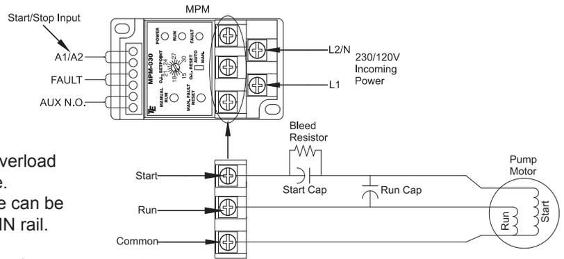
1. Verify that the FLA rating of the motor is within the overload setting shown on the top of the Motor Power Module.
