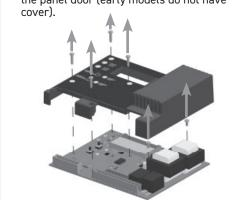
6. Install the new PCA to the panel door by using the 2 short 3/8" screws on the 2 holes on the right side of the PCA.
