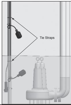
Functionally test the level measurement and ensure proper operation of the system by filling the tank.
