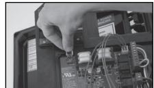
**18.** Find the end of the wiring harness that has two green terminal block plugs. Plug these into the main RK circuit board, with the 2-position plug going into the remaining 2 positions of the 5-position header, and the 4-position plug going into the 4-position header.
