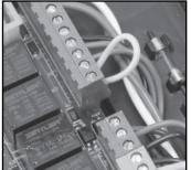
**14.** Plug the green 3-position terminal block into the new RK Series<sup>™</sup> panel 4-20mA circuit board. It will need to be placed in the top three positions of the 5-position terminal block header.
