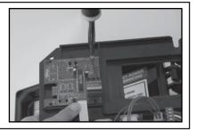
17. Plug the RK-DIB display board's ribbon cable into the main RK 4-20mA Series™ panel circuit board.
