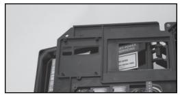
4. If no display circuit board is installed, remove the black plastic cover from the display area of the inner door.
