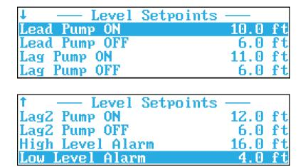
An edit screen can be brought up by pressing the selection wheel when the desired setpoint is highlighted.
