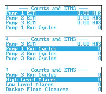
A CLEARING COUNT APPROVAL screen can be brought up by clicking the ENTER button when the desired count is highlighted. Pump ETMs cannot be cleared.
