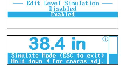
Rotate the selector wheel to make fine adjustments. To make coarse adjustments, press and hold the ◀ button while rotating the selector wheel.
