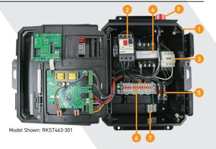
The RK Series™ Three Phase Simplex 4-20 mA continuous level sensing panel is designed to control one 208/230/460 VAC three phase pump in water and sewage installations. The protective inner door features panel operating status indicators, LCD display, control buttons and provides access to the pump motor protection switch. Panel is designed for 4-20mA input and 2-float backup control.
