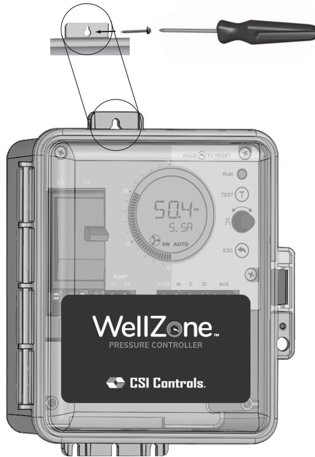
2 Drill and fasten bottom of the enclosure using appropriate anchors.
