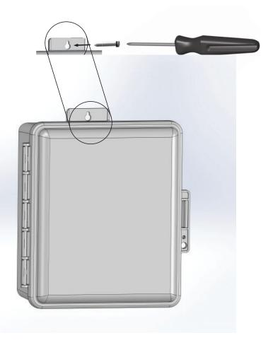
**2** Drill and fasten bottom of the enclosure using appropriate anchors.
