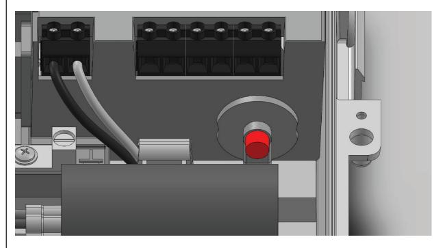
There is an additional overload (OL) protection device on 2HP and 3HP control panels. This OL device is for the protection of the START Circuitry and is located below the terminal blocks.
